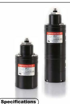
Snap Acting Relay is the device which is usually used with an air tank, converts an air flow direction and moves the valve to the fail-safe position when the signal air pressure is lower than the set air pressure. Also, it has a fail-freeze function to help the valve stay at the last position on the loss of a supply air pressure.
