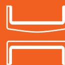
**Reduced port sleeves.** Tapered in the middle to restrict flow. Used for precise flow control and throttling.
