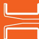
**Cone sleeves.** For more precise flow modulation than full bore designs, with less restriction than reduced port sleeves. Used to control flow rates, reduce velocity smoothly, and minimise turbulence.
